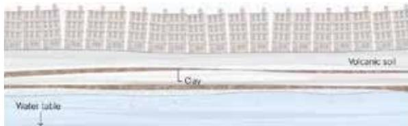
Fig. 3: Diagrammatic representation of the regional subsidence mechanism in Mexico City (Kimmelman).
