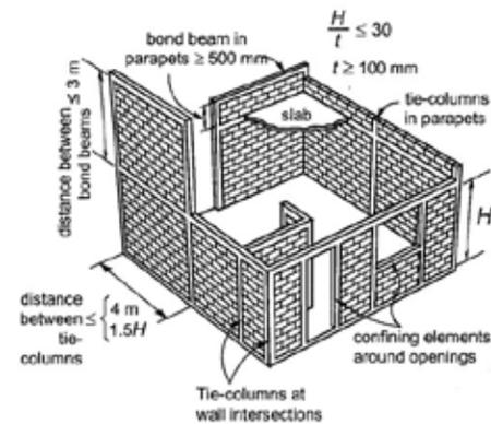
Fig. 7: Typical confined masonry construction (Alcocer, et al.).
