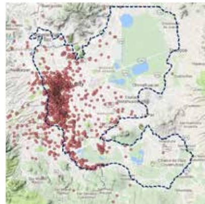
Fig. 2: Overlay of damaged buildings during the M7.1 Central Mexico earthquake (red dots, Verificado19s) and extent of the lakebed soft clay and transition zones (Mexico City Building Code).
