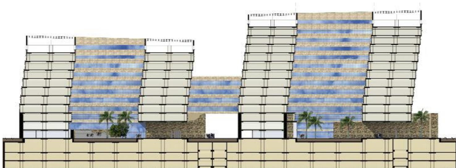
The building is stepped-up towards the south – self-shading is the result.
