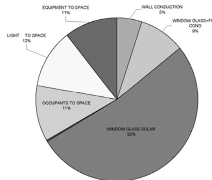
Fig 4. Typical office building cooling loads breakdown (Source; EDS, 2007)
