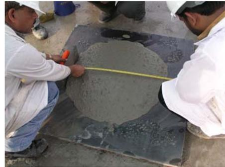
Figure 10 - SCC Conc. Flow Table Testing
