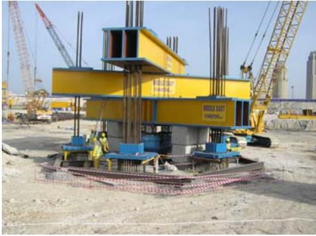
Figure 12 – Test Pile (6,000 tonnes)
