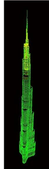
Figure 6 - 3D View of Analysis Model
