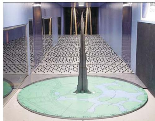
Figure 14 – Aeroelastic Wind Tunnel Model
